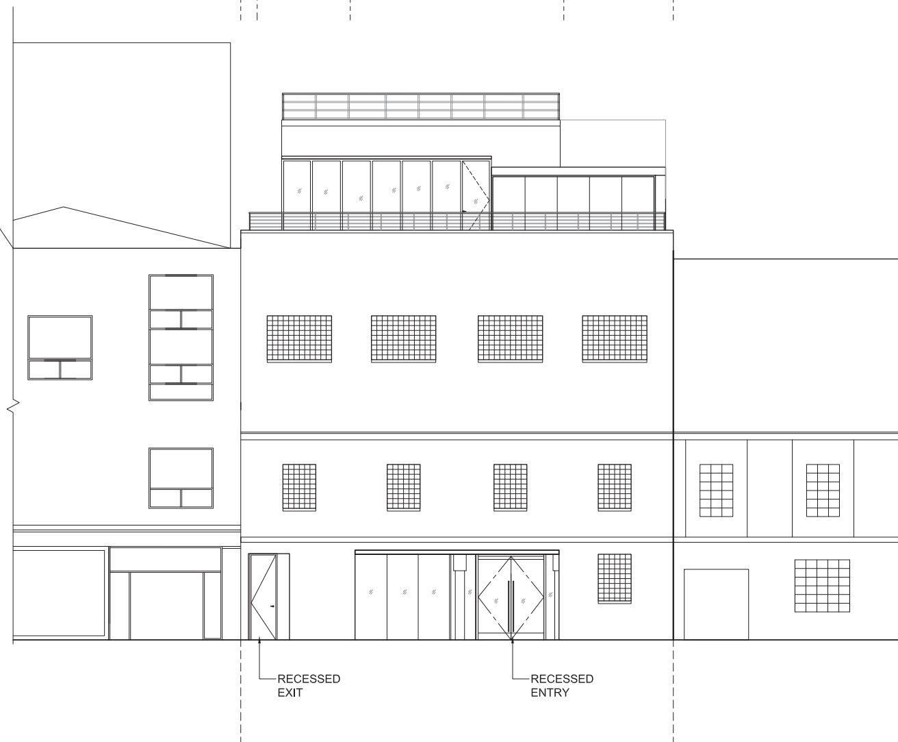
PROPOSED WEST ELEVATION 1 1/8" = 1'-0"
